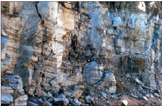
Figure 9. Wollastonite mine face, Lewis, New York. Tenor of the ore is up to 60% wollastonite. Dark streaks are pyroxene (diopside) and grossular-rich garnet.
