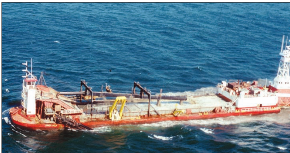
Figure 20. Trailing-arm suction hopper dredge Sandy Hook operates in lower New York Harbor to extract construction sand and gravel.
