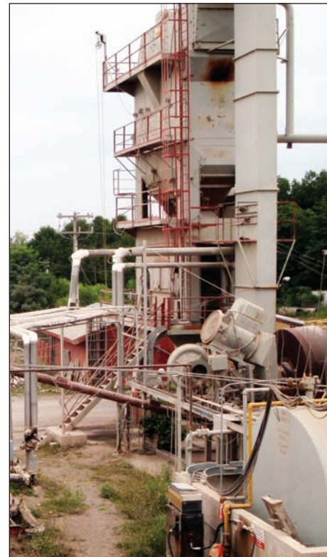
Figure 24. Baghouse dust collection system (center). Also aggregate hoppers (foreground) and hot screen and pugmill (left background). Courtesy Northern Bituminous Mix, Inc.
