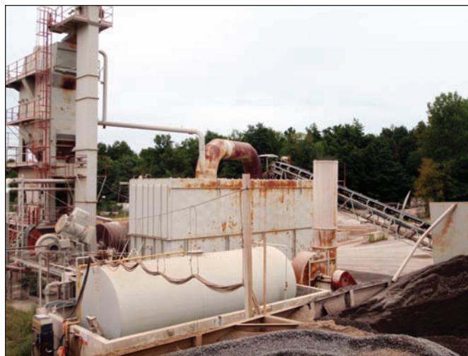
Figure 25. Hot screen deck and mill of batch-type hot mix asphalt plant. Baghouse also shown (left center). Courtesy Northern Bituminous Mix, Inc.
