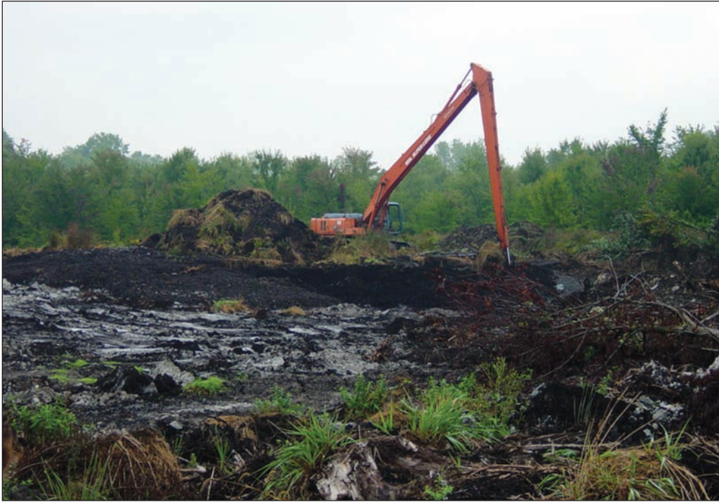
Figure 6. Peat mine, Columbia County, New York. Organic-rich muck (peat) is mixed with manure and sand to make potting soil. White material is marl.
