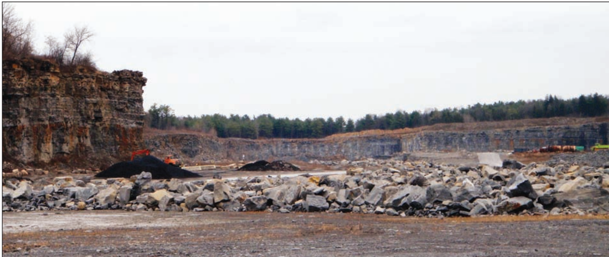
Figure 13. Typical crushed stone quarry. Dolostone units mined here are typically the Tribes Hill Formation. Courtesy Callanan Industries, Inc.
